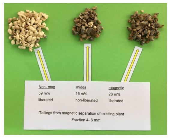
Figure 12-32 Products of magnetic separation (tailings Mix 4.0 – 6.0 mm) after separation with Permroll lab separator.
