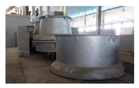
Figure 12-22 Electrical kiln
