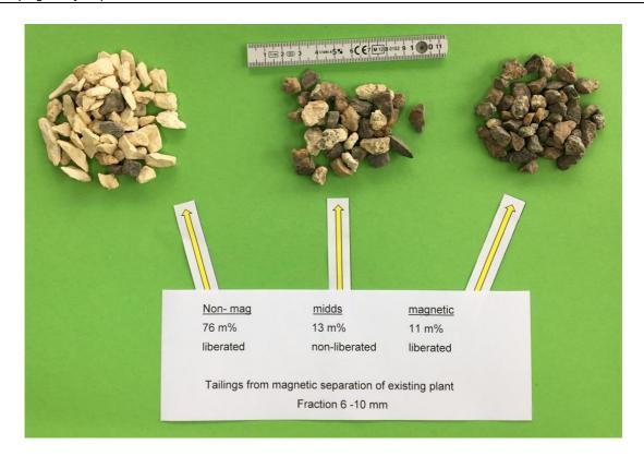
Figure 12-31 Products of magnetic separation tailings (mix 6.0 – 10.0 mm) after manual selection
