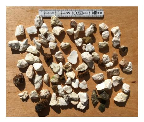
Figure 12-34 Non-magnetic (magnesite) product from magnetic separation in processing plant, 15 – 20 mm
