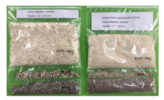
Figure 12-28 Products of magnetic separation of fraction 1.0 – 2.0 mm 0.5 – 1.0 mm mm (screw olassifier overflow)
