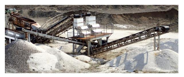
Figure 12-7 Screening and magnetic separation section of the processing plant
