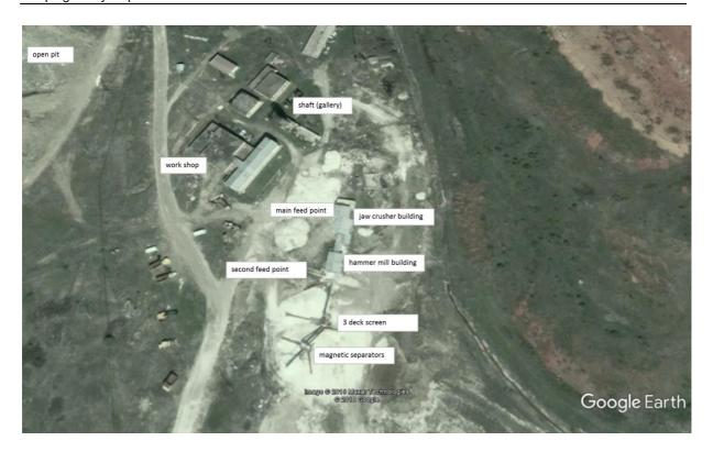
Figure 12-4 Magnesite dry/wet processing plant, location identified during site visit March 2019 (based on source: Google Earth image from 12.04.2018)
