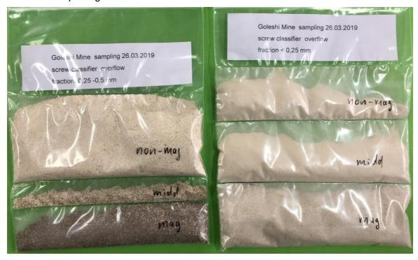
Figure 12-29 Products of magnetic separation of fraction 0.25 - 0.5 mm < 0.25 mm mm (screw classifier overflow)
