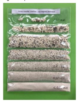
Figure 12-26 Fractions (PSD) of screw classifier overflow
