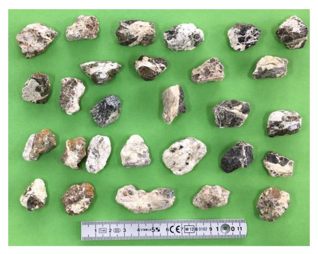
Figure 12-33 Example for non-libarated particles
