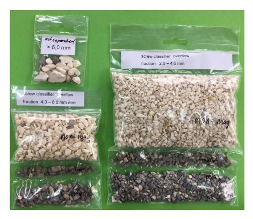
Figure 12-27 Products of magnetic separation of fraction 4.0 - 6.0 mm and 2.0 - 4.0 mm (screw classifier overflow)
